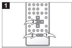
During playback, press either the Search ▶▶ button **①** or Search**◄** ■ button **②** to move the DVD forward or backward at double (x2) speed to locate a specific section. Repeatedly press these buttons and the speed will increase to x4, x8, x16 and resume normal playback.
